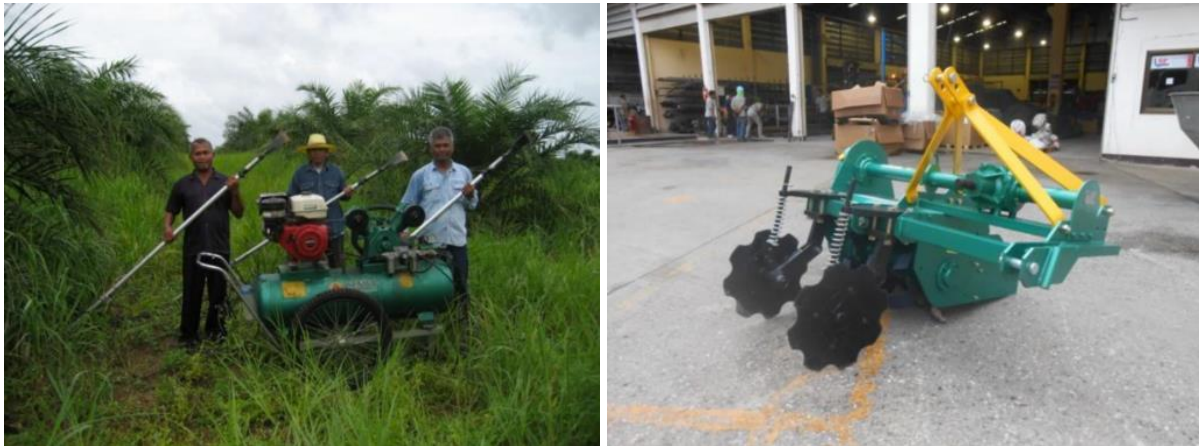
Figure 4: Development of Pneumatic Harvesting Tool for Palm Oil Industry (left) and Inter-Row Cultivator for Rice Plantation Industry in Thailand (right) (Source: Khaehanchanpong, 2018 [10])
