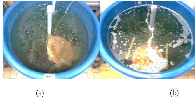
Figure 1: Water and biofloc condition of a) Micro-bubble (MB) and b) Large bubble (LB) tanks.
