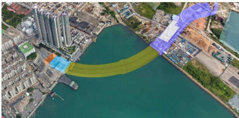
Figure 1: CKR-KTW Submerged Tunnel located at Kowloon Bay
