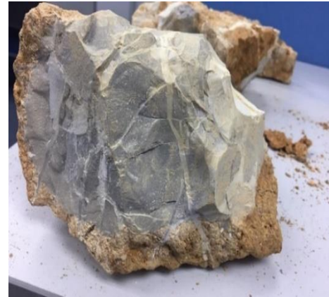
Plate 9: Treated Excavated Soil Block
