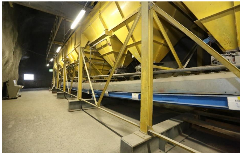
Plate 3: Underground concrete batching plant at the Hagerbach Test Facility in Switzerland
