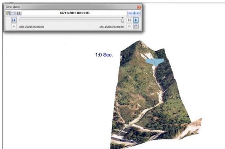
Plate 10: The simulated landslide occurred on the slope (circled). The debris flow simulation (arrowed) was computed by application of the Smoothed Particle Hydrodynamics.
