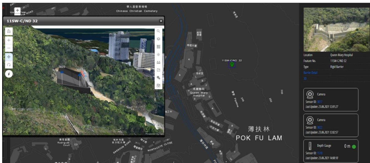
Plate 2: Integrated with BIM data, IoT sensors, 3D mesh model, and 3D digital terrain model with 3D building and infrastructure objects, the smart barrier 11SW-C/ND 32 was shown in the Smart Barriers System.
