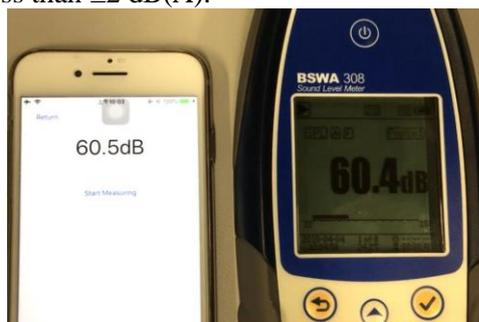
**Plate 3:** Set-up for noise calibration
