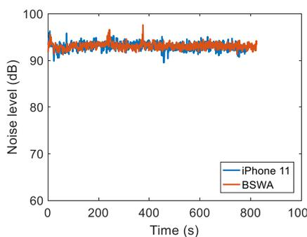
**Figure 8:** Noise level recorded by iPhone 12 and sound level meter
