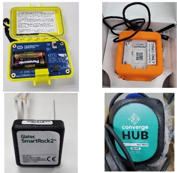
Plate 11: Four brands of temperature sensors used (top left: Command Center; top right: LumiCon; bottom left: SmartRock; bottom right: Converge)
