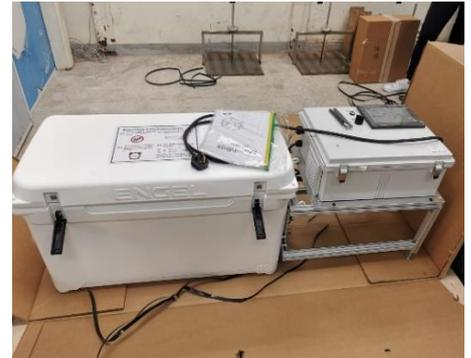
**Plate 9:** Set-up of temperature matched curing (TMC) system
