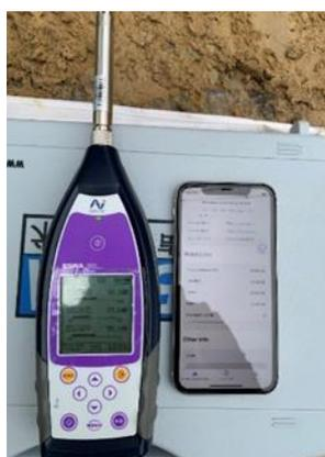
**Plate 6:** Noise measurement by iPhone 11 and sound level meter
