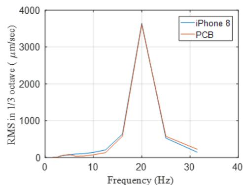
**Figure 2:** Comparison of RMS velocity in 1/3 octave band spectrum at 20 Hz excitation between iPhone and PCB accelerometer
