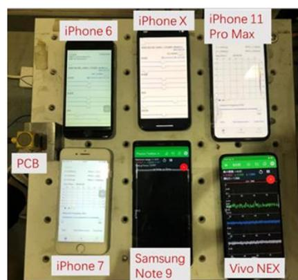
**Plate 2:** Calibration test of various smartphone models on a shaking table
