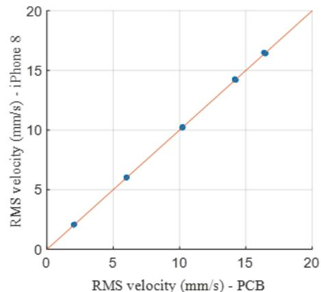
**Figure 4:** Comparison of RMS velocity at 25 Hz excitation between iPhone 8 and PCB accelerometer
