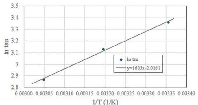
**Figure 11:** Plot of natural logarithm of τ values versus inverse of curing temperature
