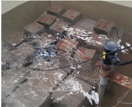
**Plate 7:** Water curing of concrete cubes in temperature control tank
