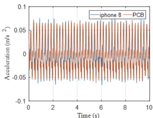
**Figure 1:** Comparison of acceleration at 4 Hz excitation between iPhone and PCB accelerometer
