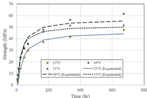
**Figure 10:** Comparison of actual and computed compressive strength
