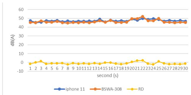
**Figure 5:** Comparison of noise level recorded by iPhone 11 and sound level meter
