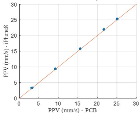
**Figure 3:** Comparison of PPV at 25 Hz excitation between iPhone 8 and PCB accelerometer
