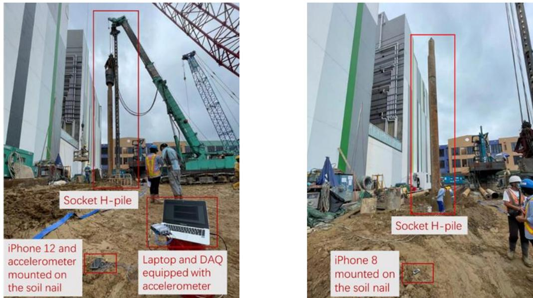
(a) Set-up for iPhone 12, accelerometer and soil nail
