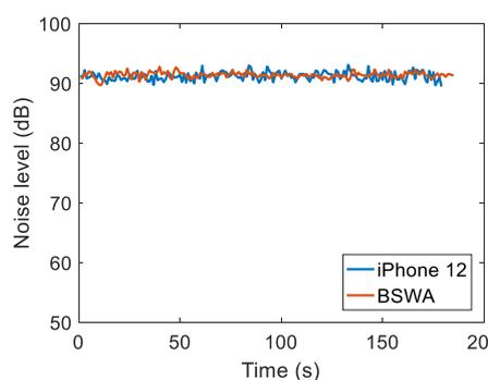
**Figure 9:** Noise level recorded by iPhone 11 and sound level meter
