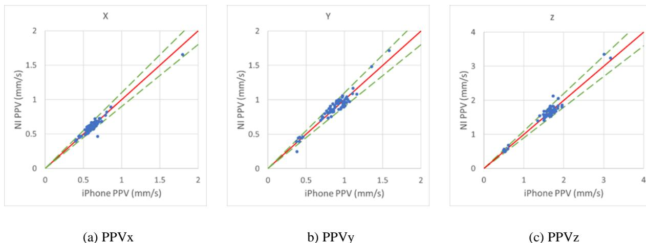
**Figure 7:** Comparison of PPV between iPhone 12 and accelerometer
