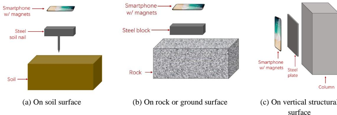
**Plate 4:** Set-up for smartphones on different types of surfaces
