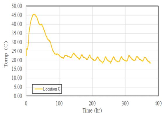
**Figure 15:** Temperature development profile at Location C recorded by Command Center sensors
