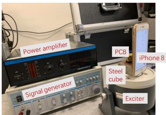
**Plate 1:** Set-up for vibration calibration
