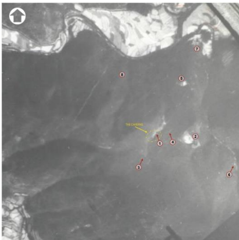
Plate 1: Aerial photograph in 1924. The cavern atrium, tailings dumps, open cast and numerous shafts and remnants of old terraces are evident.
