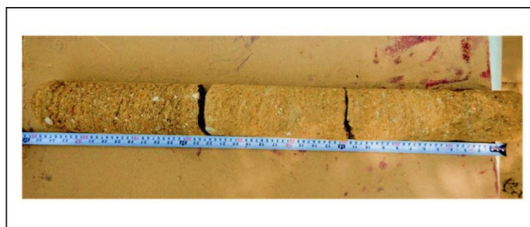
Plate 5: Samples recovered using the tailor-made core sampling method
