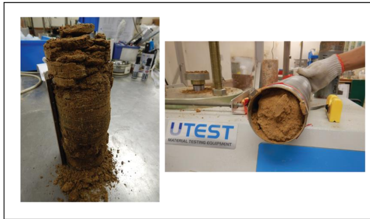
Plate 3: Poor quality of core sample with 3% cement content
