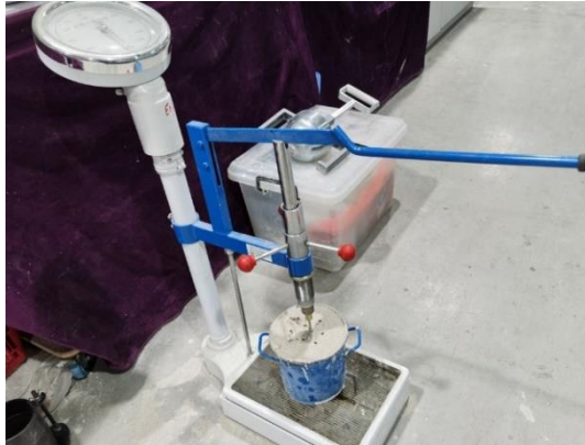
Figure 10: Hardening time testing apparatus in NAMI laboratory
