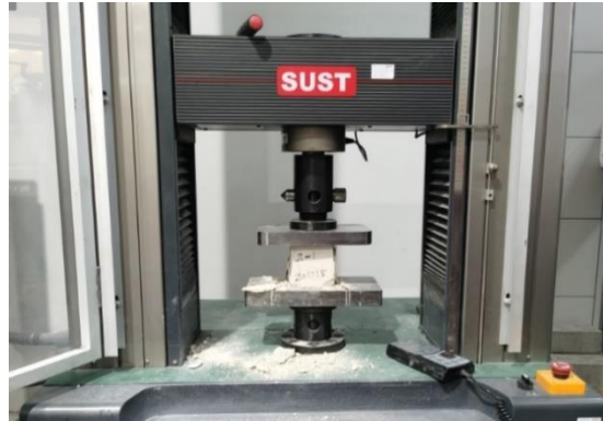
Figure 12: Sample for compressive strength testing
