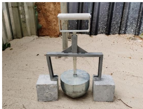
Figure 11: “Kelly-ball” test conducted on site
