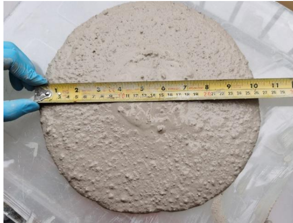
Figure 9: Measurement of flowability on site
