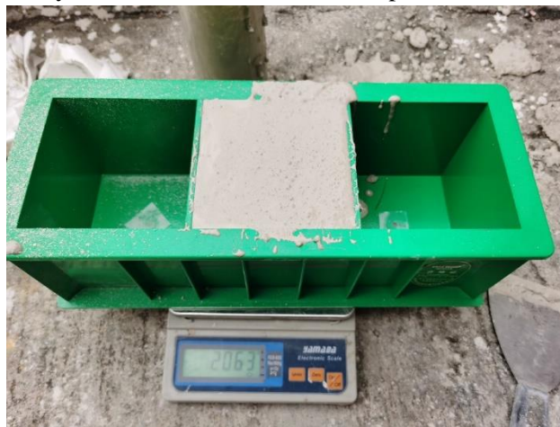
Figure 8: Measurement of wet density on site
