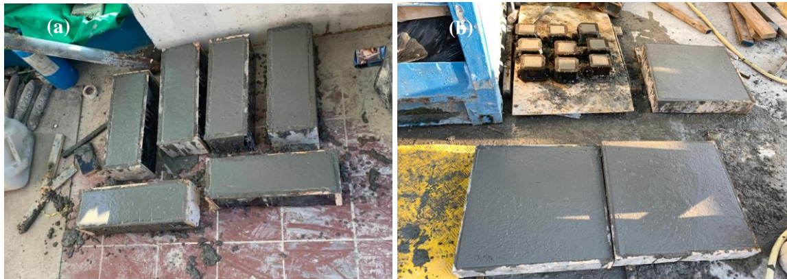
Figure 7: The fresh VRSC (a) prisms, and (b) cubes and panels
