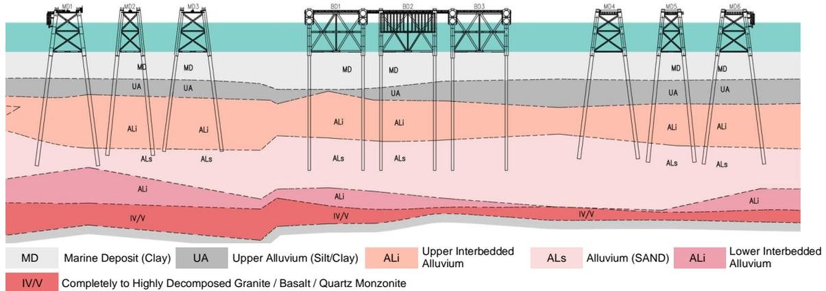
**Figure 4:** Geological Condition Over the Jetty Site
