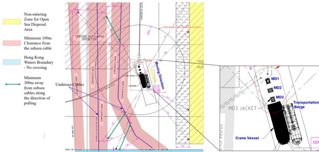
**Figure 9:** Marine Installation Constraints
