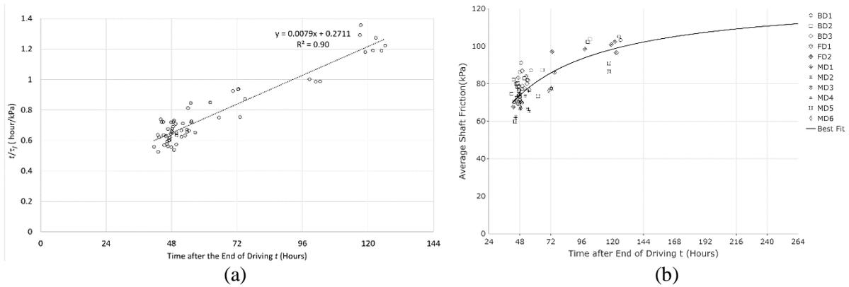
**Figure 7:** Shaft Set-up Behaviour (a)  $t/q$  vs.  $t$  and (b) average shaft friction vs. time
