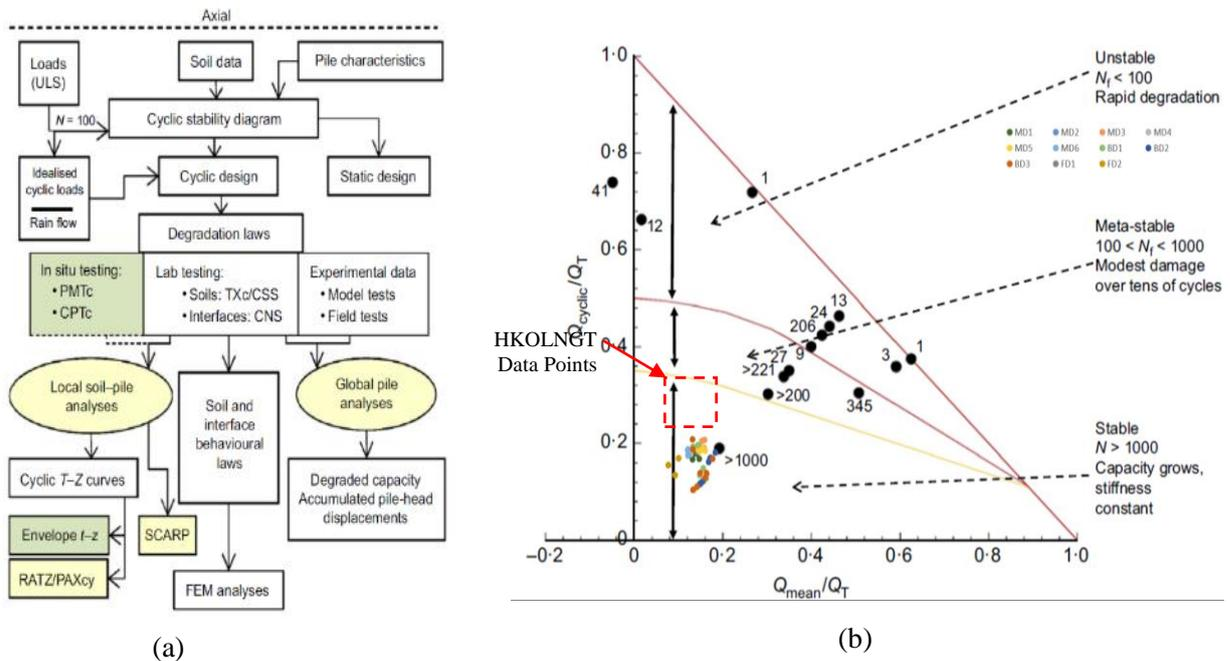
**Figure 6:** SOLCYP Workflow Process for Use in Design of Pile to Carry Axial Pile Loading (Extracted from Jardine (2020)); and (b) Interaction Diagram Developed at Dunkirk test Site (Jardine and Standing 2012, Jardine 2020) with Data Points at HKOLNGT Added
