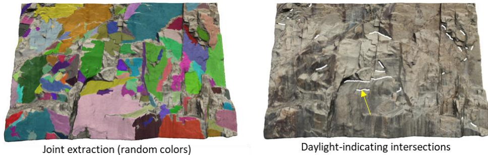
Figure 10: Results of joint extraction and search for potentially adverse daylight-indicating intersections (yellow arrow: invalid intersection)
