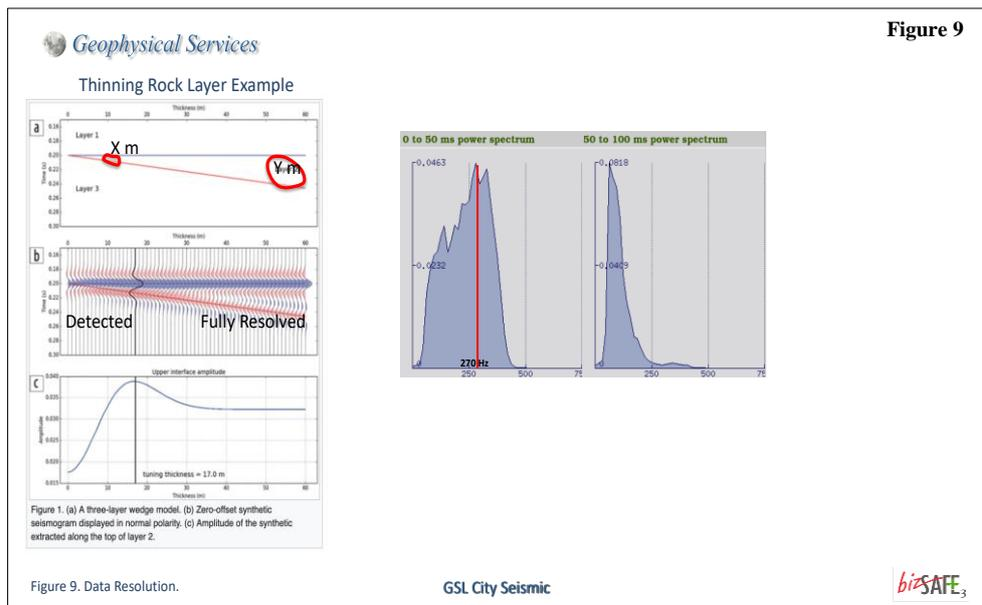
resolution and detection is also displayed. Given a peak frequency of 270 Hz, cobbles or boulders of hazardous size are assumed to be resolvable in the tunnel path.
