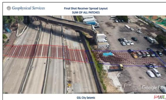
Figure 14; Post-Plot diagram showing each and every shot point and receiver points across the entire survey area
