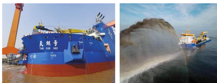
Figure 1: Tian Kun dredging and blow-filling ship
