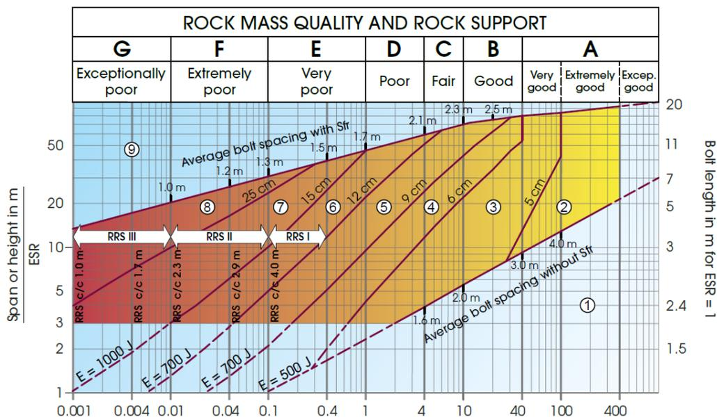
Figure 3: The Q-system rock support chart (NGI, 2015)
