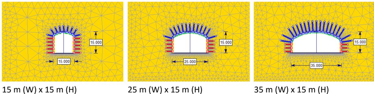
**Figure 7:** Finite element models for caverns with different span
