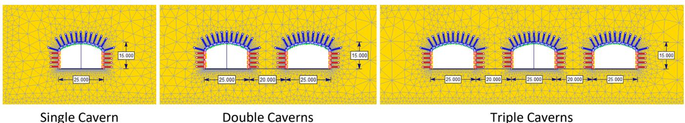
**Figure 8:** Finite element models for caverns with multiple parallel excavations
