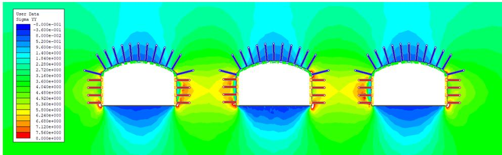
**Figure 9:** Superimposed vertical stress ( $s_{vv}$ ) concentration at rock pillars in FEM
