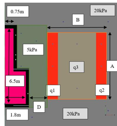
**Figure 8:** Typical scheme for Plant Load Cases (Y-Panel), Plaxis 3D
