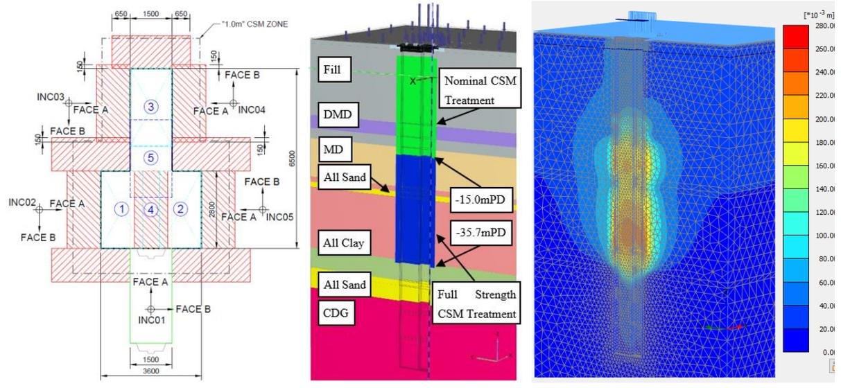
**Figure 13:** Y-Panel diaphragm wall excavation sequence and CSM ground treatment on plan and section views
