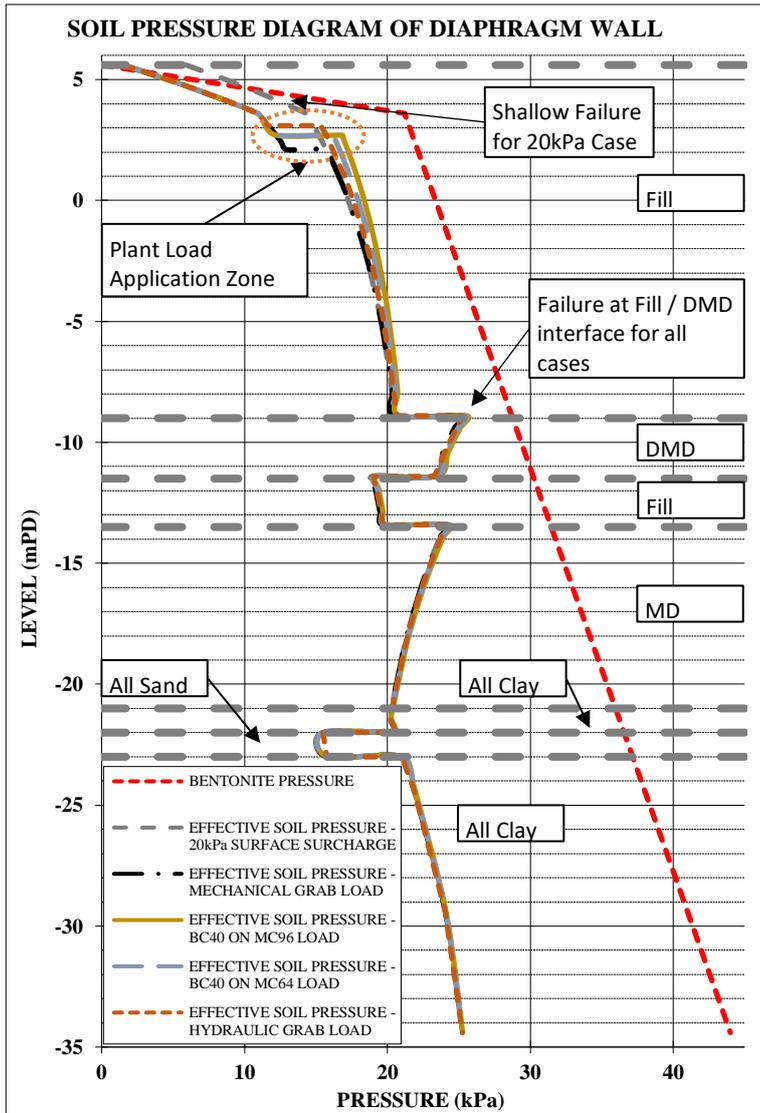
Figure 9: Pressure Diagram of Diaphragm Wall Trench
