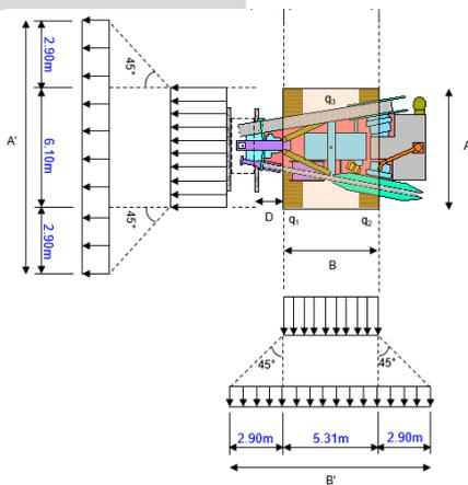
**Figure 6:** Load Case D for Pressure Balance Method
