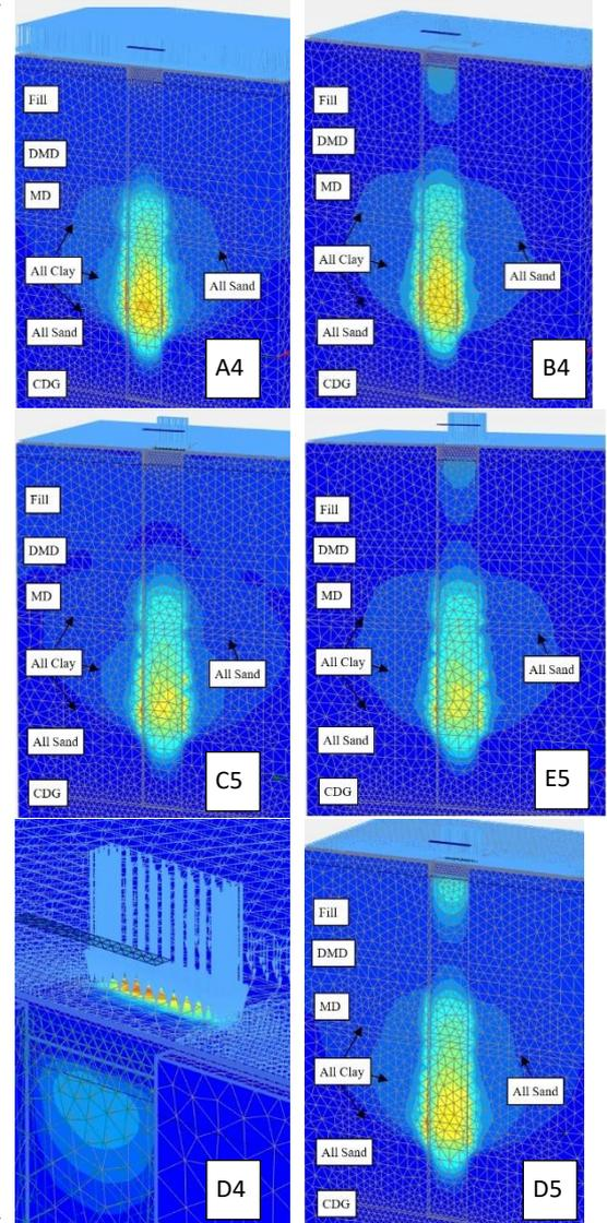
Figure 10: Failure Mechanism for all Load Cases
