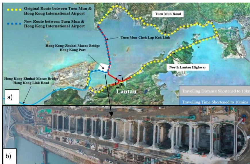
**Figure 1:** a) Tuen Mun Chek Lap Kok Link Project Location, adapted from [www.hzmb.hk/eng/about\\_tmckl.html](http://www.hzmb.hk/eng/about_tmckl.html) (Accessed on the 31/03/2021); b) Hybrid ELS Scheme, courtesy of Dragages Bouygues Travaux Public JV
