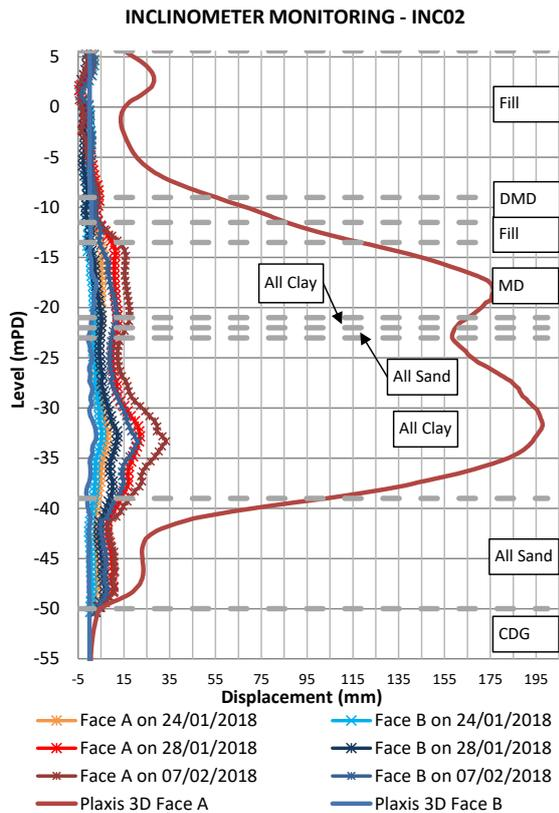
**Figure 17:** Long Panel Incliner Monitoring Results
