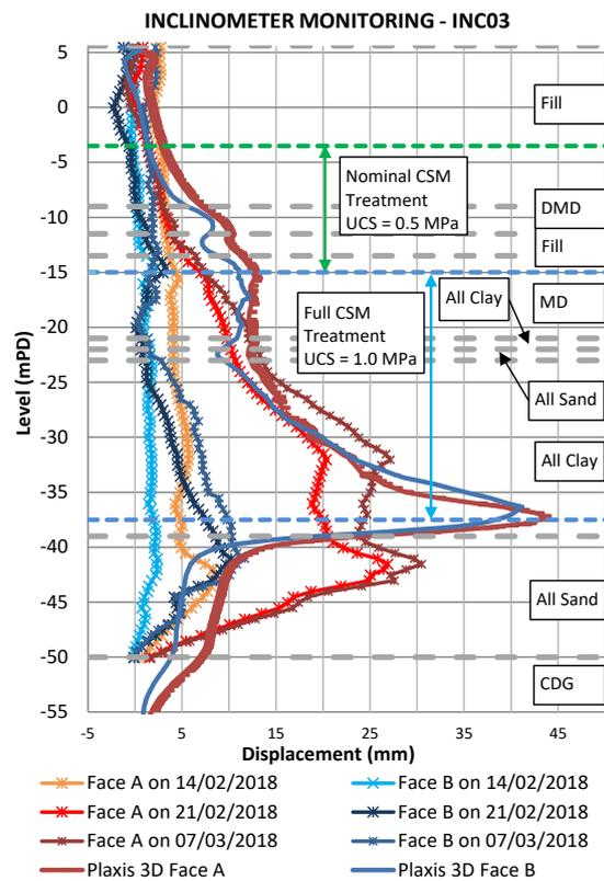
**Figure 18:** Y-Panel Incliner Monitoring Results
