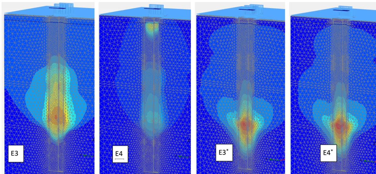
**Figure 15:** Y-Panel Failure Mechanisms without CSM
