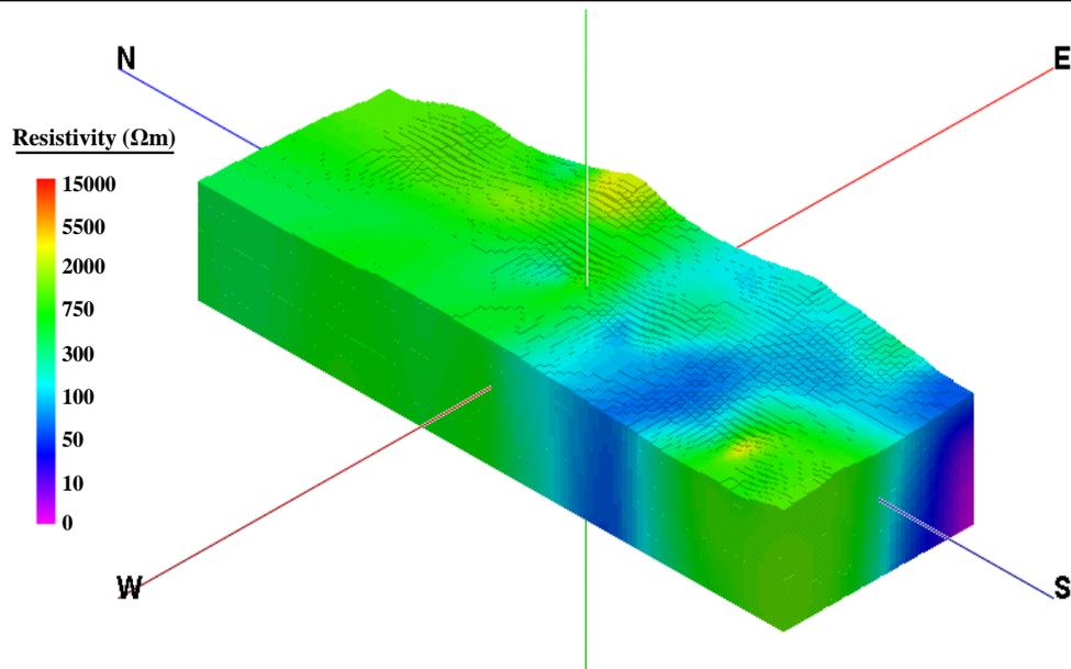
Figure 4: 3D resistivity model of the study area
