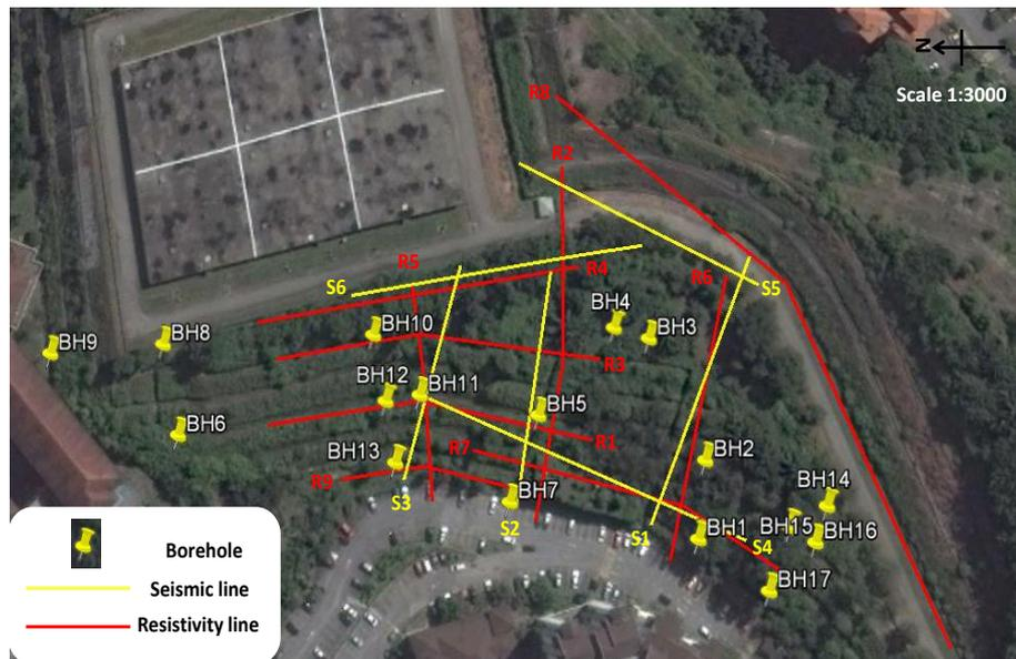
**Figure 1:** Location of boreholes, resistivity lines and seismic lines
