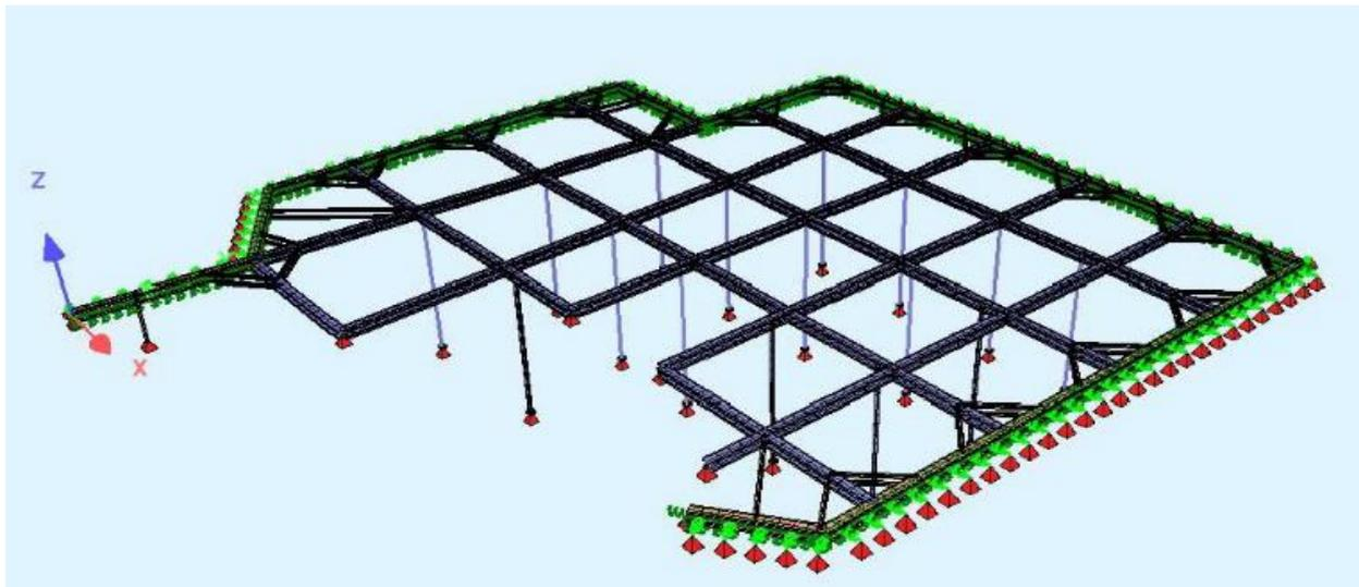
**Figure 8:** 3D Structural Model for Strut Design
