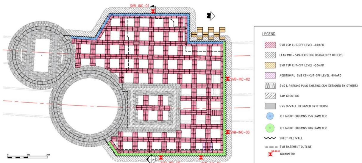
Figure 7: Ground Improvement Layout Plan
