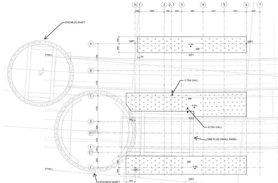
**Figure 3:** Layout Plan of Original Piling Scheme
