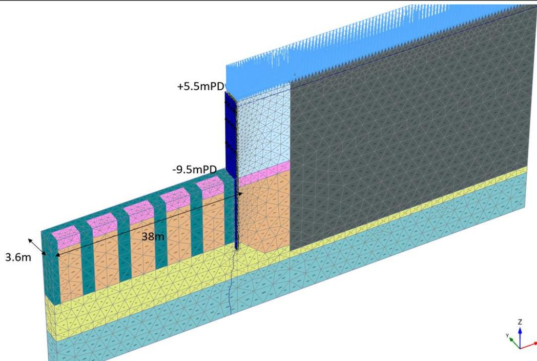
Figure 9: 3D FE Model for Temporary Excavation Design
