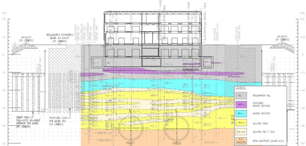
Figure 5: Geological Section
