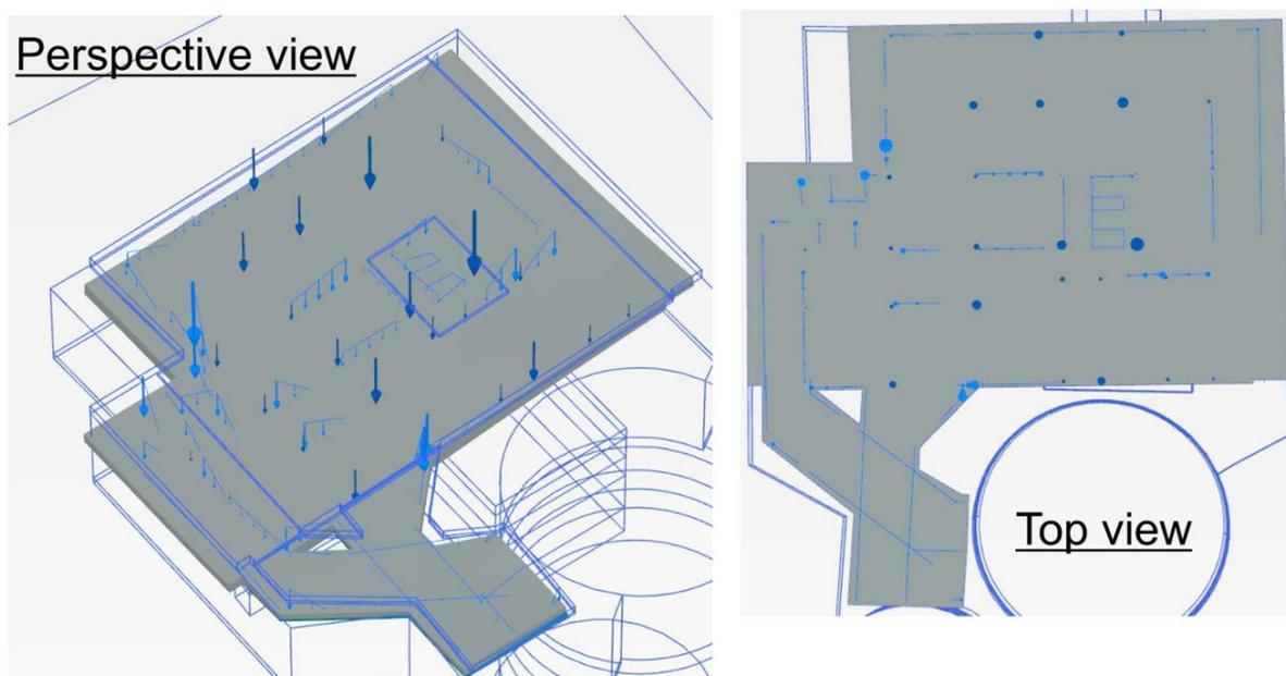
Figure 10: 3D FE Model for Foundations Design
