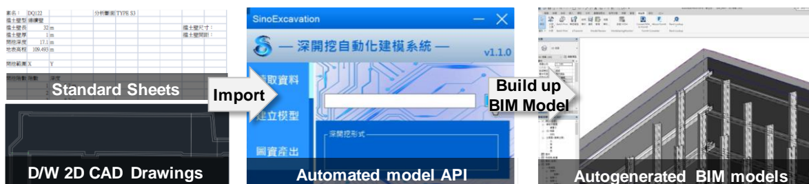
Figure 2: The process and interfaces of SinoExcavation auto-generate BIM models
