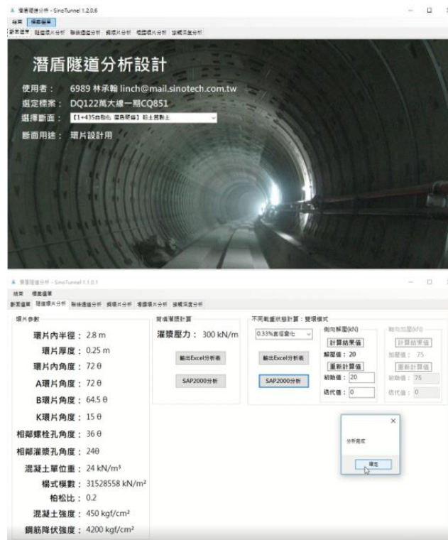
Figure 5: The Winform interface, which can automatically call SAP 2000 to conduct the iteration itself
