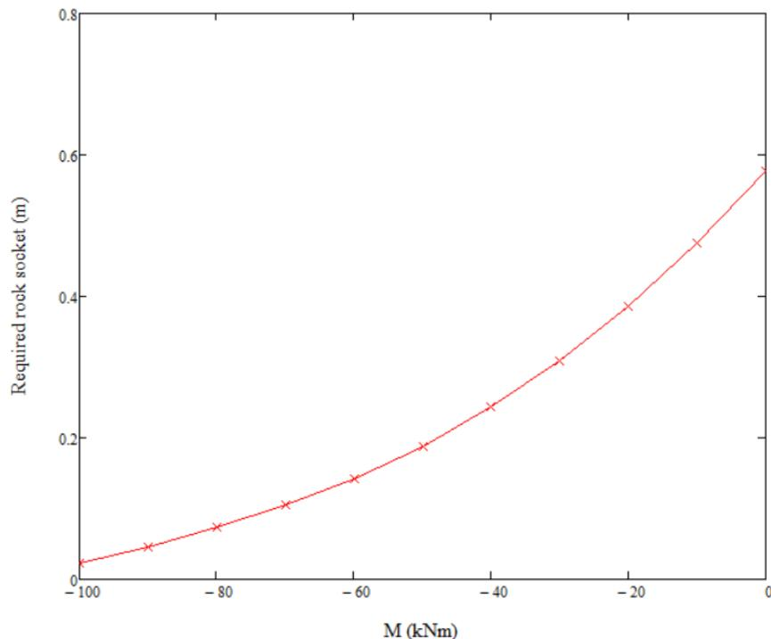
**Figure 8:** Required socket length for selected combinations of  $M$  and  $V$  for Stage 2 works
