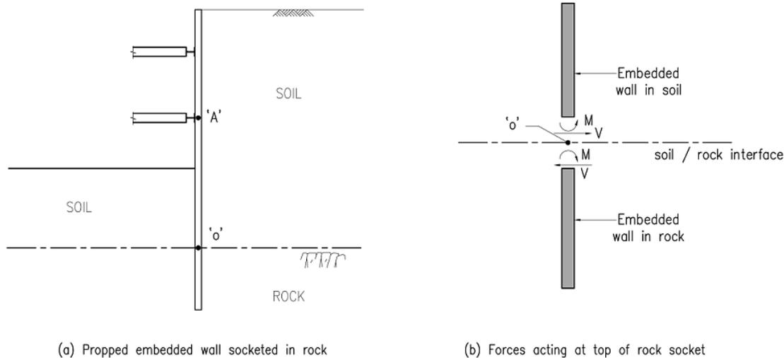
**Figure 4:** Analysis of a propped embedded wall partially embedded in rock
