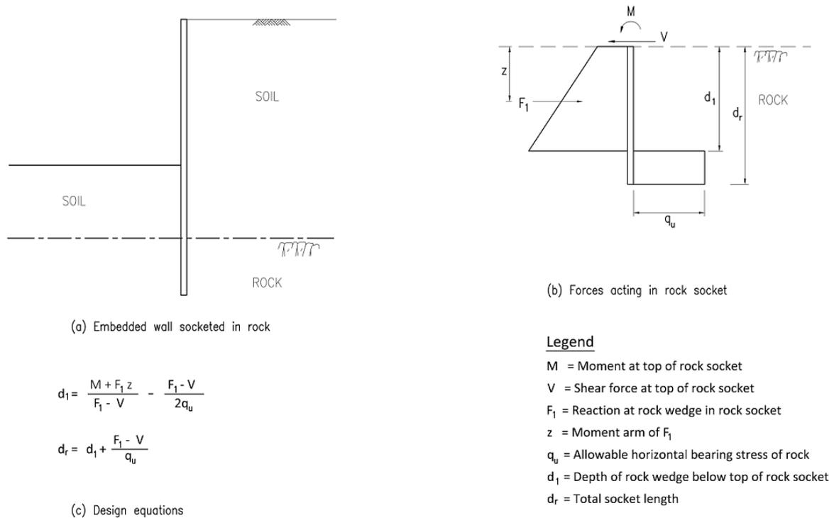
**Figure 3:** Design equations for determination of rock socket length based on Geoguide 1 (2<sup>nd</sup> Edition)
