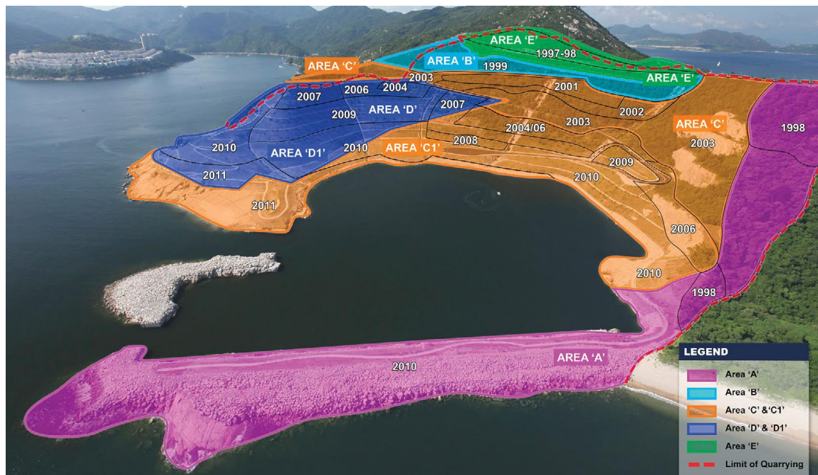
Figure 2: The project was divided into five phases e.g. Area E (1998), Area B (1999), Area A (1998), Area C (2003) and Area D (2011). Retrieved from https://www.concrete.hk/system/files_force/assets/document/hkila_2012_sq4_low_res.pdf
