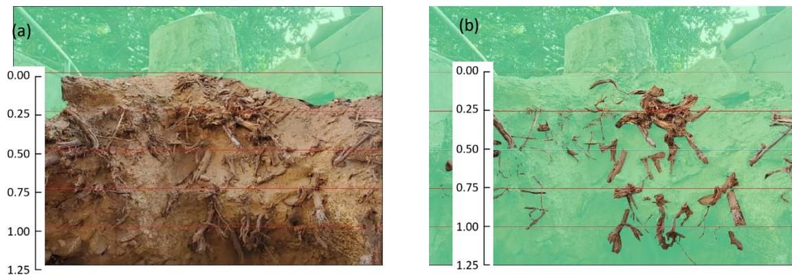
**Figure 2:** (a) rooted soil photograph taken from a 30m high species with a DBH of 750mm up to 1.25m depth
