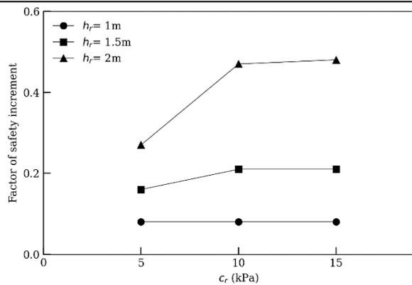
**Figure 5:** Factor of safety increments for the root zone with respect to bare slope against sliding
