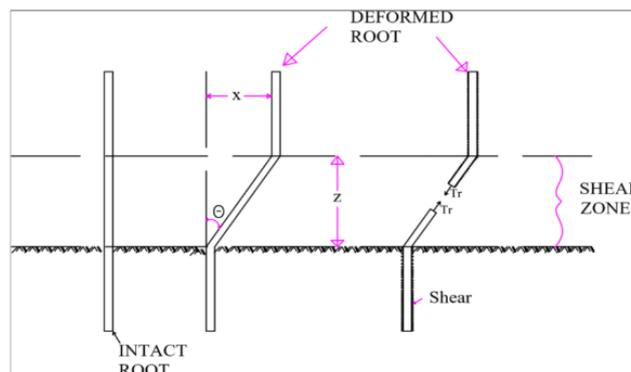
**Figure 1:** Fiber breakage model (adapted from Tsige et al., 2019)
