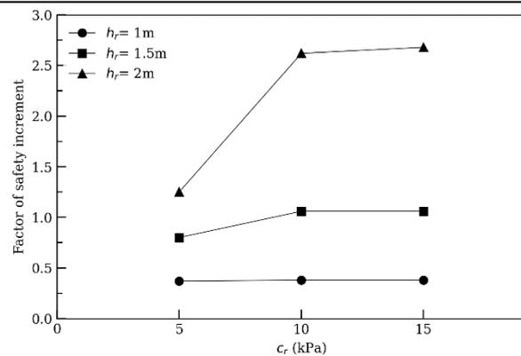
**Figure 6:** Factor of safety increments for the root zone with respect to bare slope against overturning
