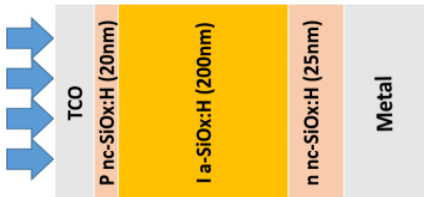
Fig.1: Schematic structure of a-SiO x :H based thin film solar cell.
