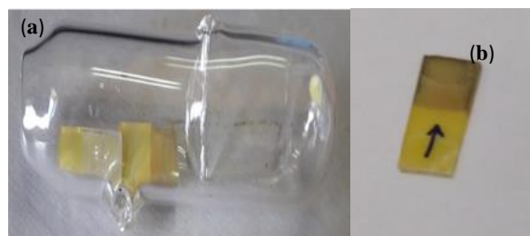
Fig.1: Photography images of (a): the films in the capsule, and (b): sample after annealing under sulfur atmosphere.
