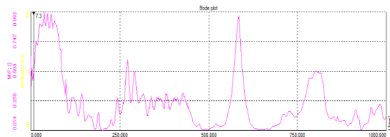
Fig.27 MIF graph of Cracked Beam (CL300mm CD 8mm)
