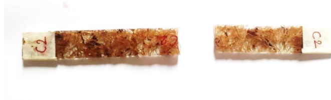
Figure6: Impact Test Specimens after Fracture
