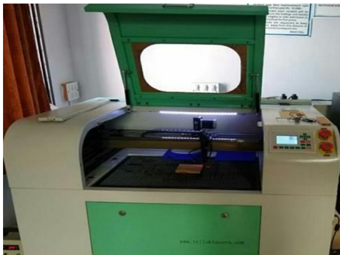
Figure 2: CO 2 Laser Machining Set-up
