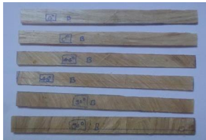
Figure 7: Specimen with 40/60 composition before tensile test
