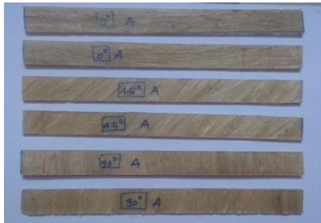
Figure 6: Specimen with 30/70 composition before tensile test
