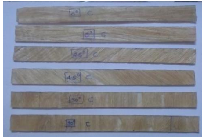
Figure 8: Specimen with 50/50 composition before tensile test
