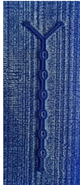
Figure 6: Fabricated microchannel or mold with Elliptical Obstacles
