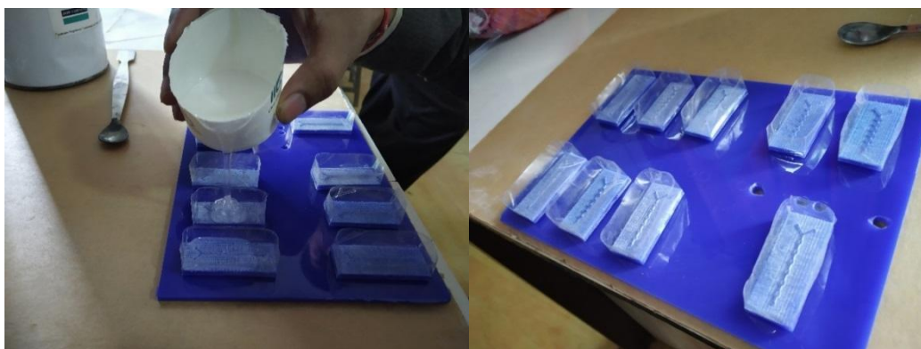
Figure 8: Pouring of PDMS during fabrication of Microchannels using Soft Lithography
