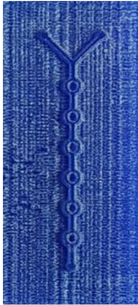
Figure 5: Fabricated microchannel or mold with Circular Obstacles
