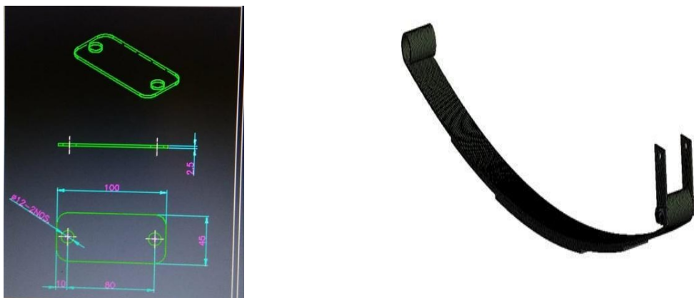
Figure 1: Meshed model of Leaf Spring Fig.2 Base line of Shackle plate
