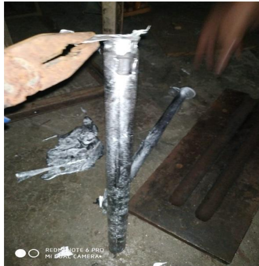
Figure 4 Rod formed after casting
