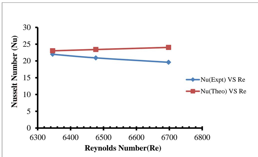
Figure 8: Nusselt Number ( $Nu$ ) and Reynolds Number ( $Re$ ) variations for inserts inclined at  $90^\circ$
