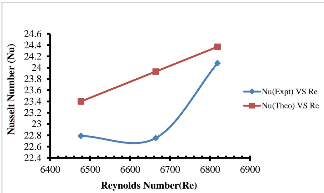
Figure 7: Nusselt Number ( $Nu$ ) and Reynolds Number ( $Re$ ) variations for inserts inclined at  $45^\circ$
