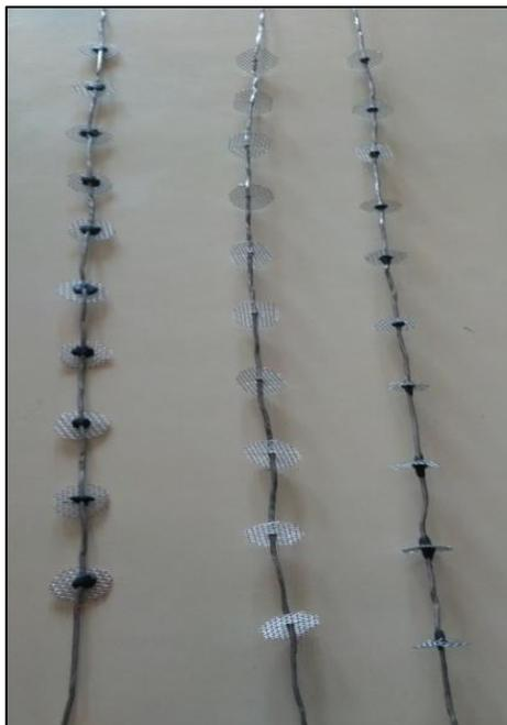
**Figure 2: Photograph of inserts inclined at 0°, 45° and 90°**
