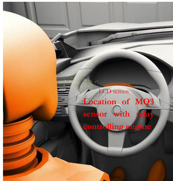
Figure 5: Sensor Installation location
