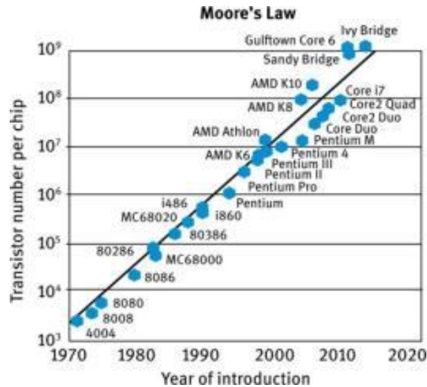
Fig 1 : Moore’s Law graph of no. of components on a chip vs year -No. of components on a chip doubles after every two years. This graph shows the most recent scenario till the year 2020 [2]
