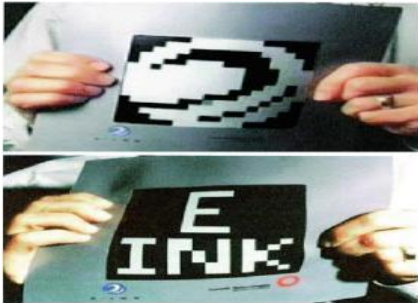
Fig.9. Shown above is an electrophoretic display. First of its kind, an OTFT display using pentacene TFT [15]
