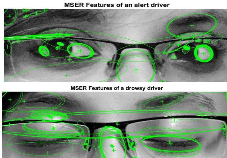
Figure 7: MSER Feature Detection of Pre-loaded Images (Open and Closed Eyes).
