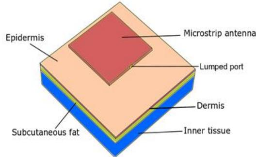
Figure 1. Schematic geometry of multilayered skin tissue model with microstrip patch antenna.
