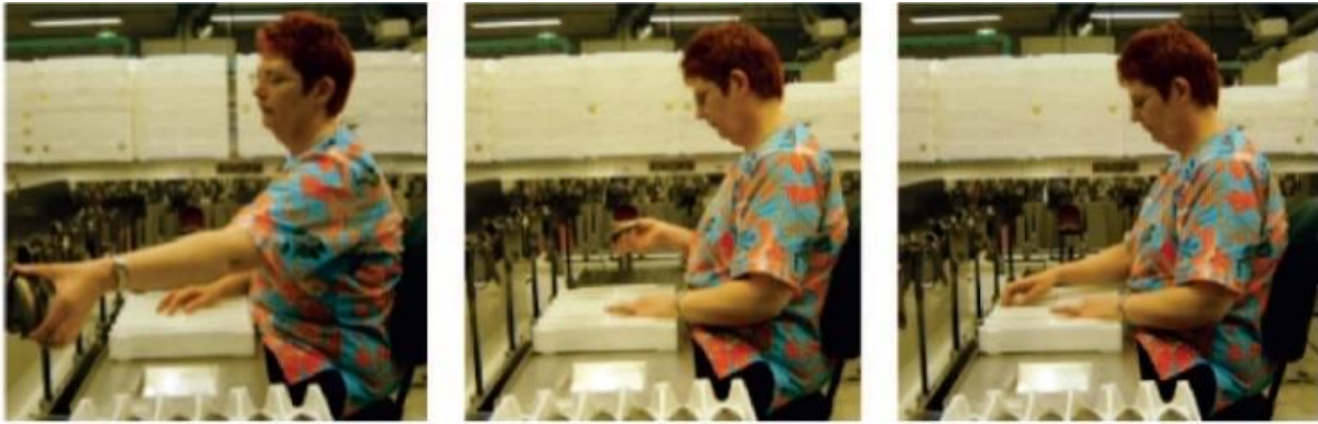
Fig. 3. Task performed in [22]. (a) picking the product; (b) visual control; (c) placing the product.
