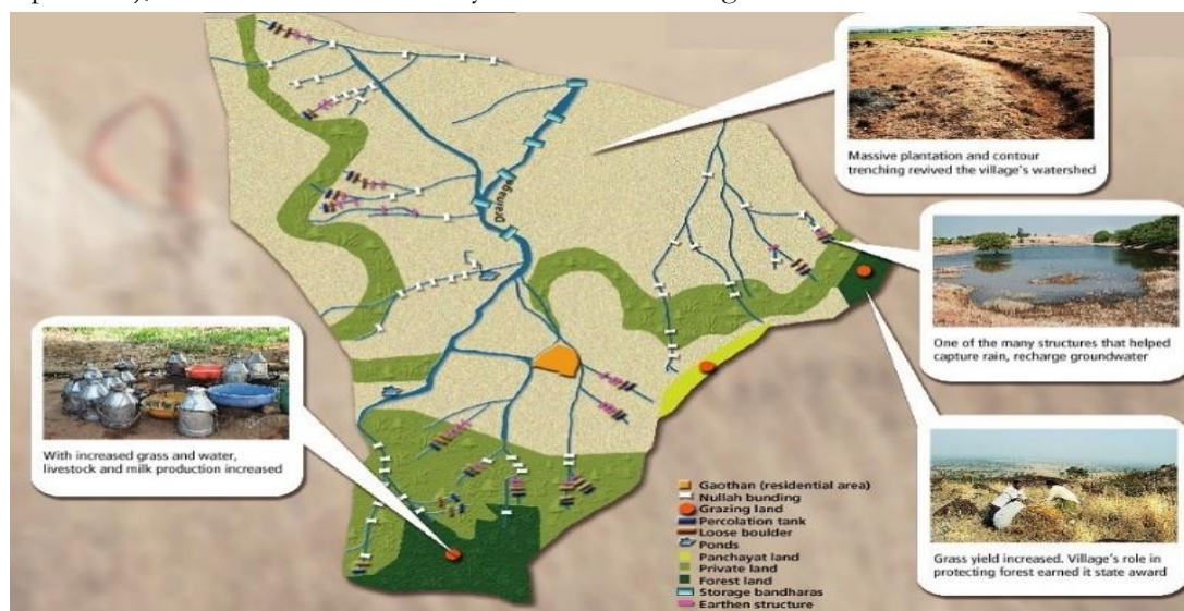
Figure 3- location of water conservation structures in Hivre bazaar till 2007 (Indian water portal, 2007)
