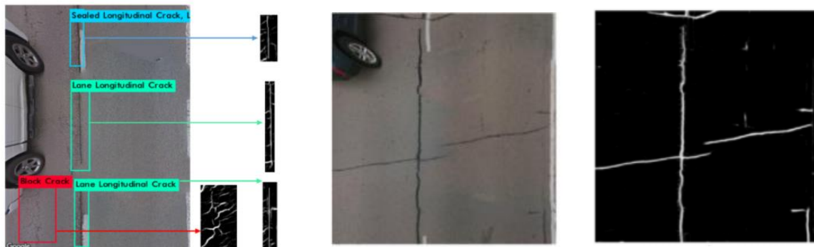
Figure. 2. Distress detection using deep learning model (H. Majidifard et. al. 2020)
