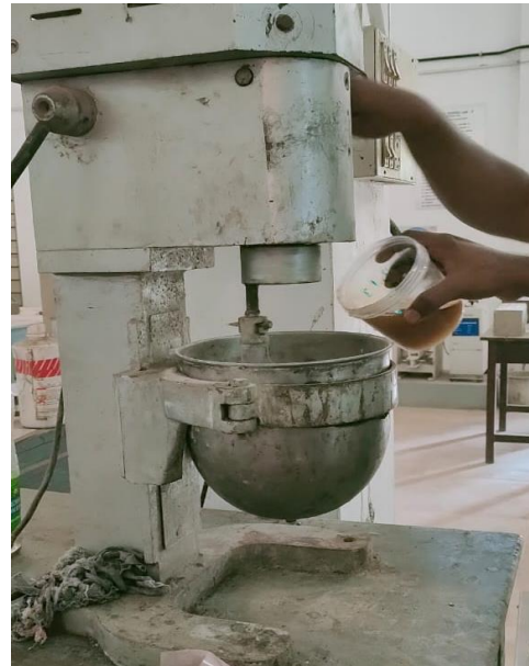
Figure 2. Preparation of geopolymer mortar using Hobart mortar mixer
