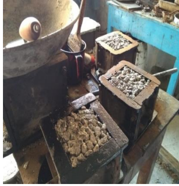
Figure 2. Cast Concrete Specimens
