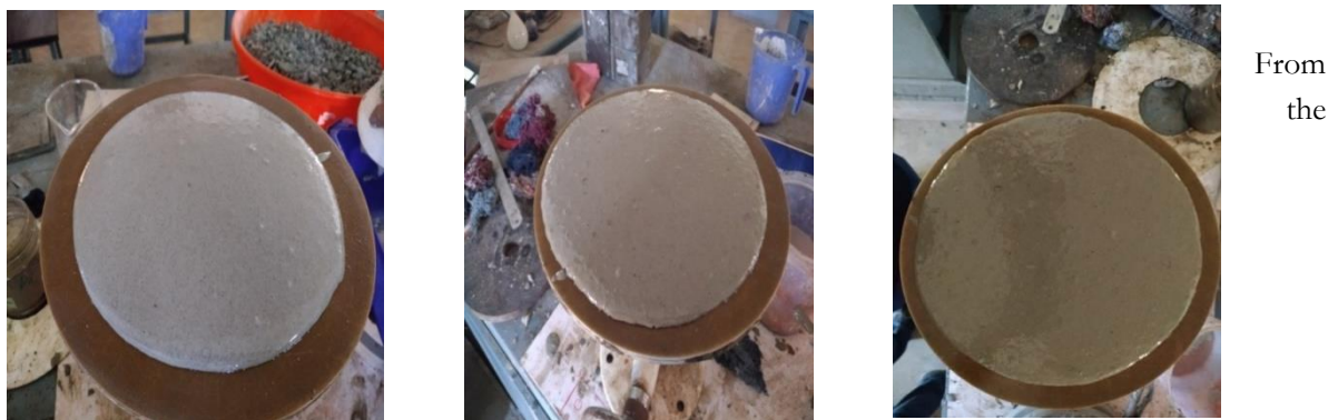
Figure 2. Flow of mix with 100% slag and a/b ratio of 0.7, 0.8 and 0.9 respectively
