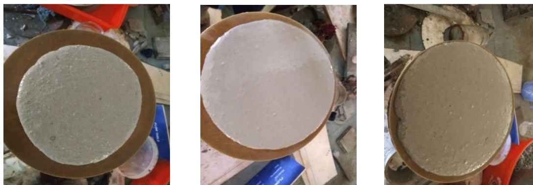
Figure 2. Flow of mix with 100% slag and a/b ratio of 0.7, 0.8 and 0.9 respectively
