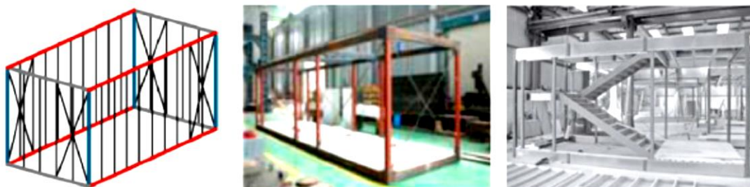
Fig. 2.1. Classification of modules in MSC (continuously supported, frame supported and non-load bearing modules respectively) (Deng et al., 2020) [6]
