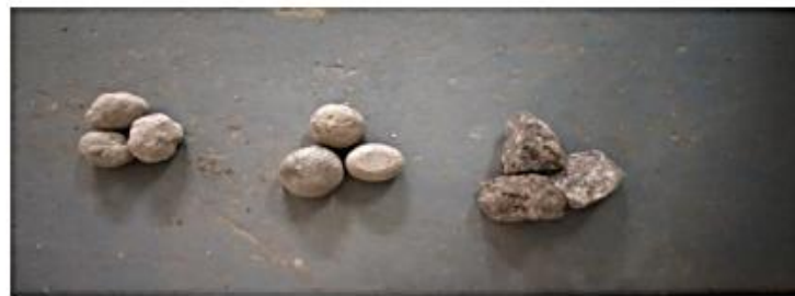
Figure 5. Comparison of shape of mix 1, mix 2 and normal aggregates
