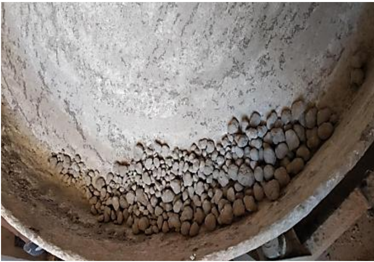
Figure 1. Fly ash pelletization in progress
