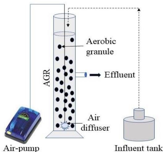
**Figure 1.** Schematic diagram of aerobic granular reactor (AGR)
