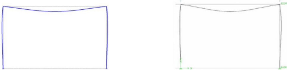
Figure 7. Frame deformation (PLAXIS and ETABS) (Ali Akhtarpour and Mahbubeh Mortezaee 2016)
