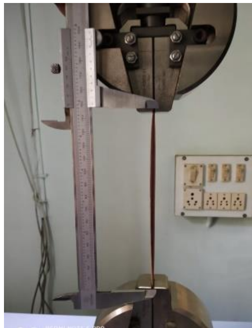
Figure. 2 Tensile strength measurement arrangement
