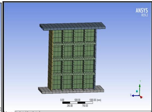
**Figure 2. Meshed structure of SPSW**
