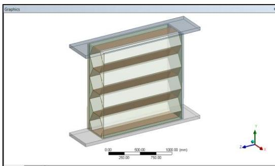
**Figure 10. ASSW with honeycomb core**
