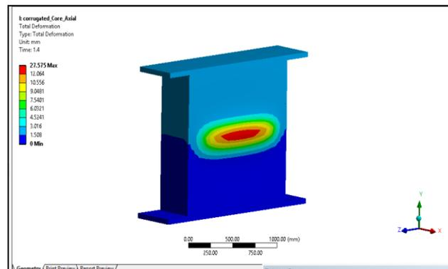
Figure 5. Deformation of ASSW with corrugated core under axial load
