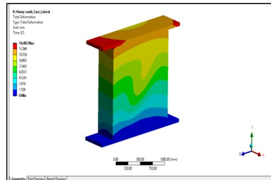
Figure 13. Deformation under monotonic load
