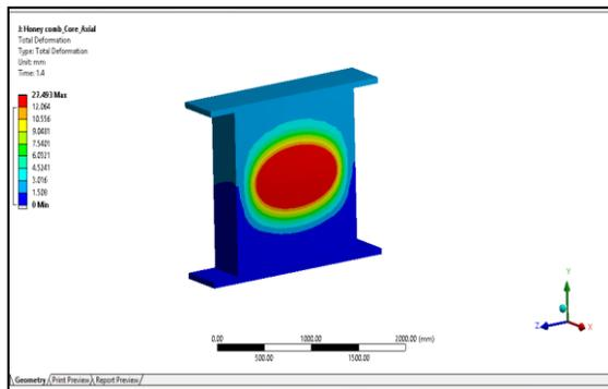
Figure 12. Deformation under axial load
