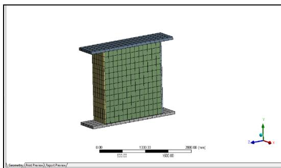
**Figure 11. Meshed structure of ASSW**
